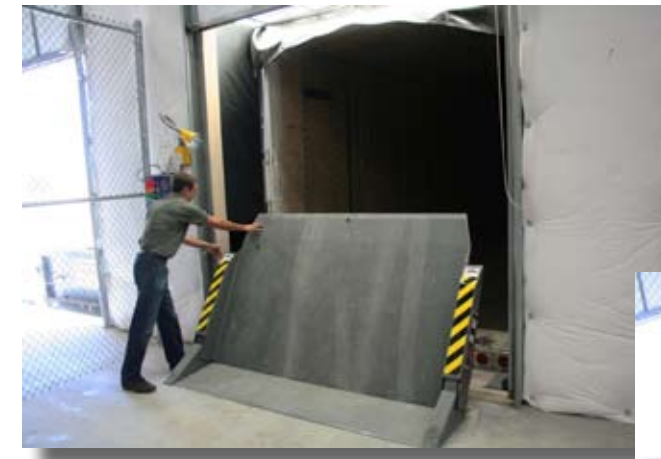
◀ Lower – A release of the lever on the LoadHog dock bridge enables it to softly lower in place to the truck trailer bed, enabling shipment of positioning arms at the Stryker manufacturing plant.
